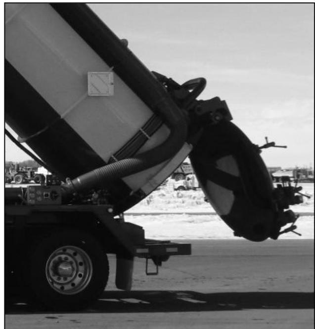
Photograph of the rear door configuration of a typical hydrovac truck. Note crush point.
