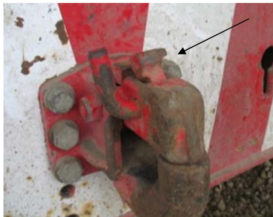
Pintle hitch in partially closed position showing latch not fully depressed
