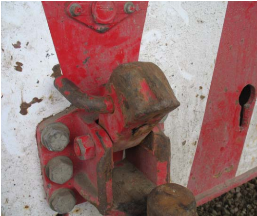
Pintle hitch in open position
